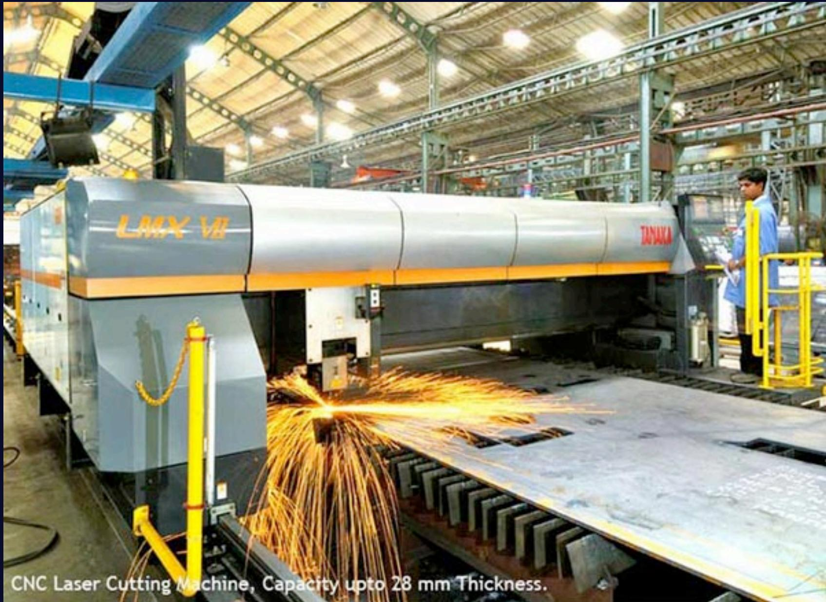
CNC Laser Cutting Machine, Capacity upto 28 mm Thickness.
